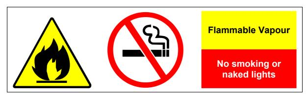
The Dangerous Substances and Explosive Atmospheres Regulations (DSEAR) apply where flammable gases are present. These regulations mean technicians must protect people, including the public, whose safety may be put at risk from fires or explosions which could occur. Guidance on technician's responsibilities under DSEAR should be taken from the HSE website, <a href="https://www.hse.gov.uk">www.hse.gov.uk</a>.
