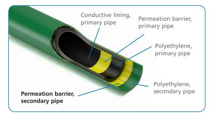
the secondary pipe wall to the environment. All double wall KPS bends, fittings and tees used in fuel product lines also have permeation protection. This best-in-class practice exceeds the requirements of the current EN 14125 standard and sets KPS apart from competing PE pipe systems that use unlined secondary containment which will permeate **120 times more.**
